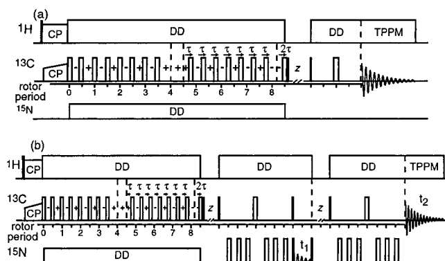
Figure 1. Pulse sequences for the CSA-filter experiment. (a) 1D: The CSA-filter pulse train consists of sixteen 180^\circ pulses phase-cycled by the xy-16 scheme. The pulses are spaced at half a rotor period apart, except for additional displacements between the eighth and ninth pulses, and between the fifteenth and sixteenth pulse. A z-filter for obtaining purely absorptive cosine-modulated signals and a Hahn echo are applied before detection. Filled rectangles: 90^\circ pulses. Open rectangles: 180^\circ pulses. The plus and minus signs represent the sign of the dynamic phases under the chemical shift evolution. (b) 2D ^{15}\text{N} - ^{13}\text{C} correlated CSA filter: The ^{15}\text{N} chemical shift evolution is inserted between the 180^\circ -pulse train and the ^{13}\text{C} detection period. REDOR is used to transfer the coherence between ^{15}\text{N} and ^{13}\text{C} .
